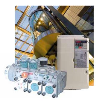
With the new L1000H inverter drive and the EV4 control valve from our partner Blain Hydraulics, YASKAWA is offering an energyefficient solution for demanding hydraulic lift applications. Upward travel is controlled by the inverter and downward travel is controlled mechanically. Other than the connection of the magnetic coils, the controller works without pressure sensors or flowmeters.
